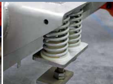
➤ Installation on springs to ensure optimum insulation with high amplitude
