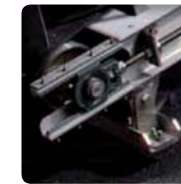
Belt tensing system
