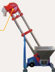
Chain or cable driving (alternative with direct gear motor)
