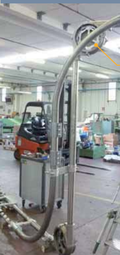
Notched angle gears wheel for discs indexing and setting in motion of the cable
