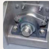
▶ Conveyor roll end bearing
