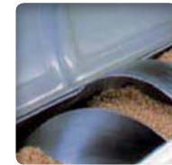
Minimum gap (flight clearance) between the tube and external screw flight (max. 5 mm.)
