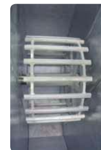
Squirrel cage design Prevents belt wear and patinating
