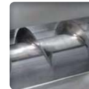
Different types of helicoil to allow the conveying of different materials
