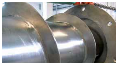
2. The screws having an oversized shaft diameter do not require intermediate bearings and have significant conveying distance. For abrasive materials, alternative to the intermediate bearing is shaft oversizing.
